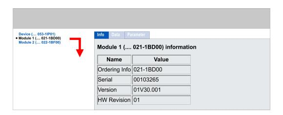
**Tab:** 'Info' Here product name, order number, serial number, firmware version and hardware version number of the according module are listed.
