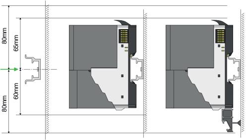
1. Mount the mounting rail! Please consider that a clearance from the middle of the mounting rail of at least 80mm above and 60mm below, respectively 80mm by deployment of shield bus carriers, exist.
