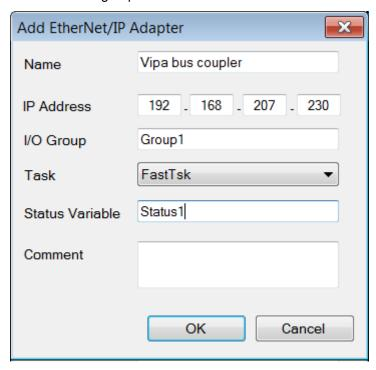
⇒ The dialog window is closed and the EtherNet/IP adapter is listed in the 'Hardware Configuration' below 'EtherNet/IP'.
