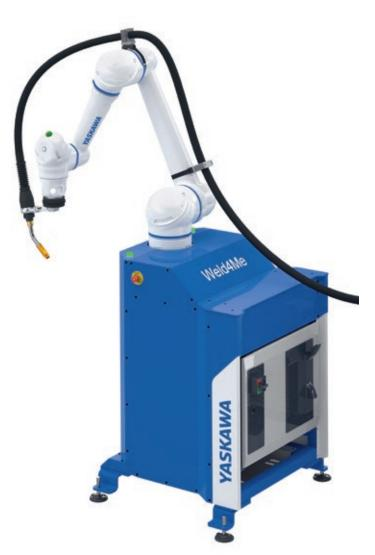
As an alternative or supplement to manual MIG/MAG welding with air-cooled welding equipment, the Weld4Me Cobot station offers all the advantages needed. It has a small footprint and is easy to move with a hand pallet truck, and it brings the consistent quality of robotic welding to your production processes.
