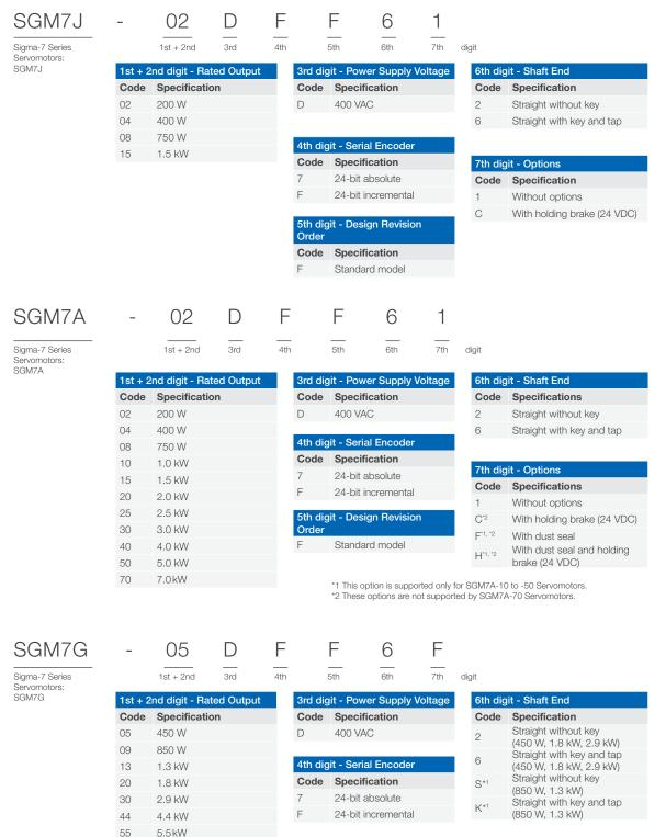
\*1 The shaft end codes are different for 850 kW and 1.3 kW Servomotors. The shaft diameter for 850 W Servomotors is 19 mm. The shaft diameter for 1.3 kW Servomotors is 22 mm.
