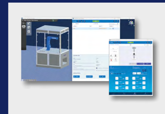
MOVAUTO Skill (Collision Free Automatic Path Planning)
