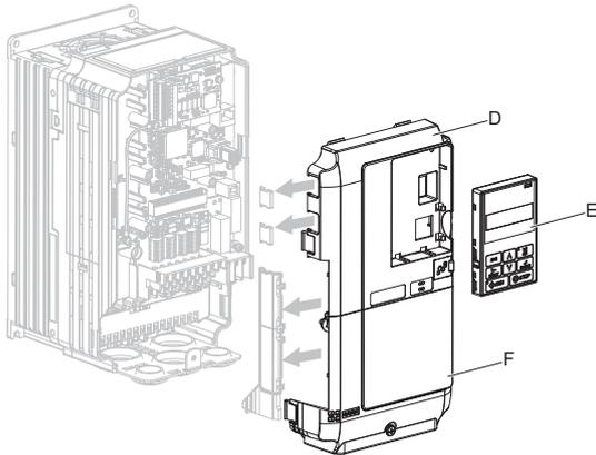
**Figure 10 Replace the Front Covers and Digital Operator**
