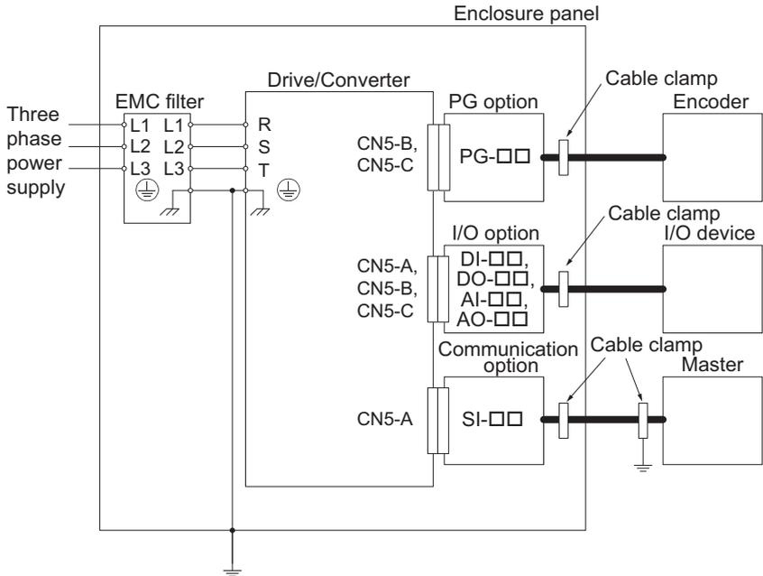
**Figure 16 Option Installation for CE Compliance**
