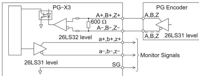
Figure 13 Interface Circuit
