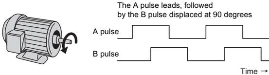
**Figure 11 Displacement of A and B Pulses**
