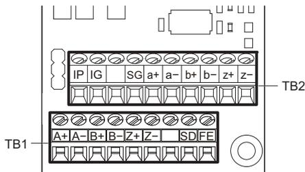
Refer to [Table 5](#) on page [26](#) for details on TB1 and TB2 terminal functions and signal levels.
