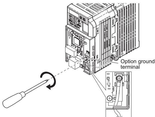
Figure 17 Connect the Ground Wire to the Option
