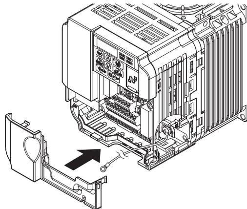
**Figure 13 Reattach the Terminal Cover**
