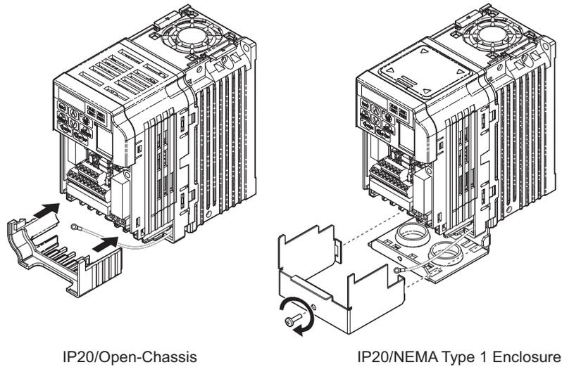
**Figure 12 Reattach the Bottom Cover**
