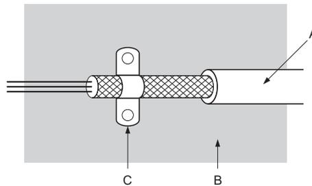
A – Braided shield cable                      C – Cable clamp (conductive)
