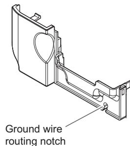
**Figure 14 Terminal Cover Ground Wire Notch**
