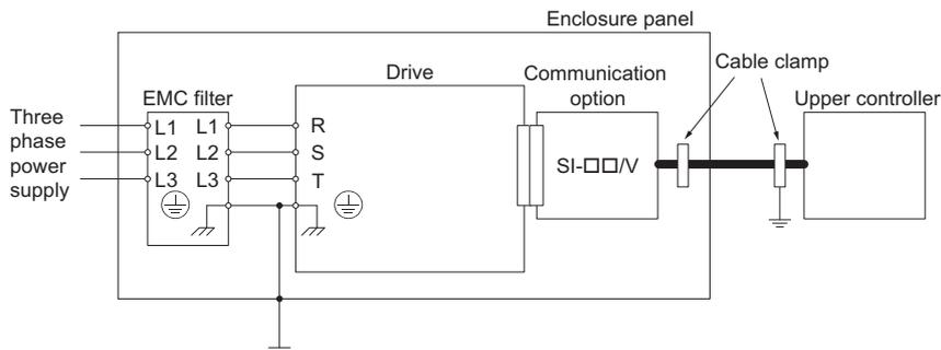
Figure 26 EMC Filter and Option Installation for CE Compliance
