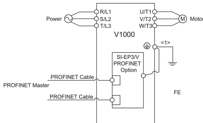
Figure 20 Wiring Diagram
