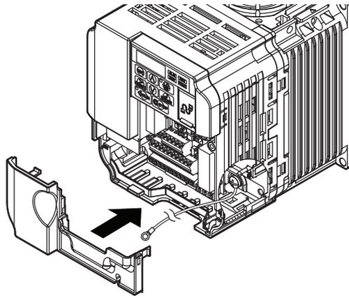
**Figure 13 Reattach the Terminal Cover**
