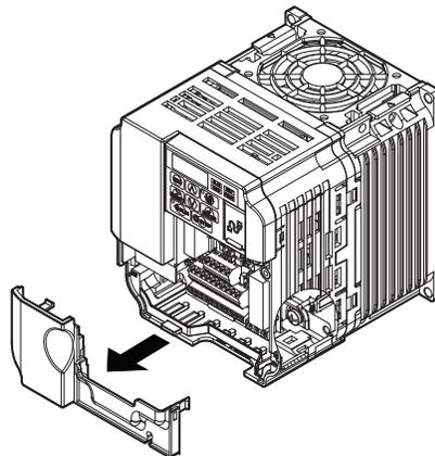
**Figure 9 Remove the Terminal Cover on an IP20/NEMA Type 1 Drive
