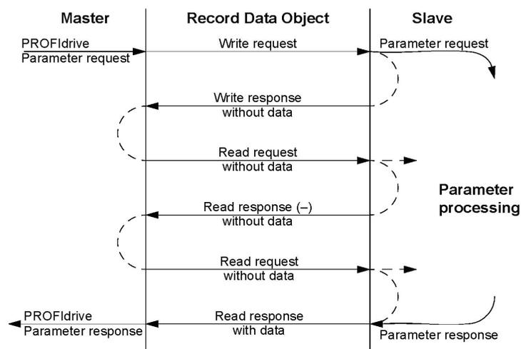
**Figure 23 PROFIdrive Acyclic Parameter Access Mechanism Structure**
