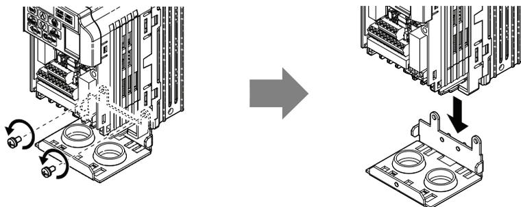
**Figure 10 Remove the NEMA Type 1 Conduit Bracket**
