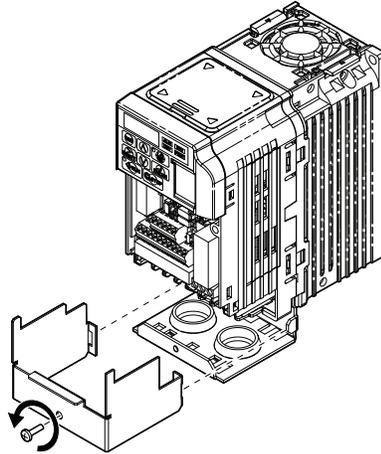
**Figure 8 Remove the NEMA Type 1 Terminal Cover**
