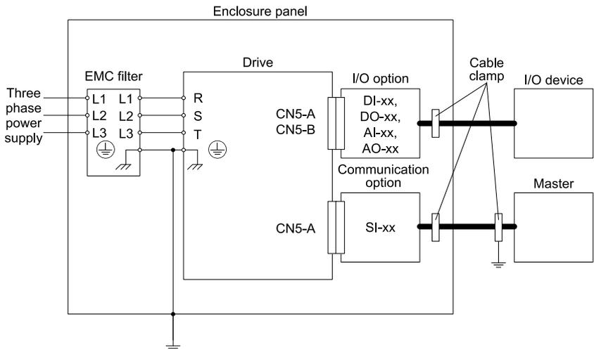
**Figure 10.4 Option Installation for CE Compliance: FP605**
