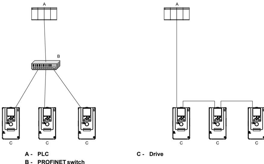
**Figure 5.23 Prepare and Connect Communication Cable Wiring**
