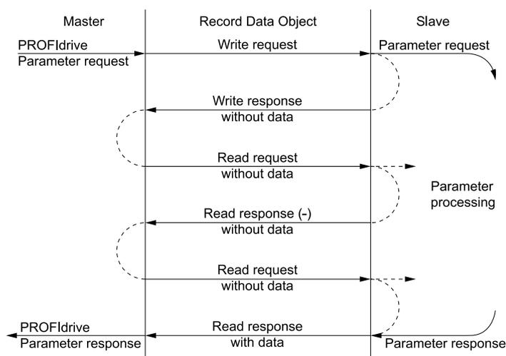
**Figure 8.1 PROFIdrive Acyclic Parameter Access Mechanism Structure**
