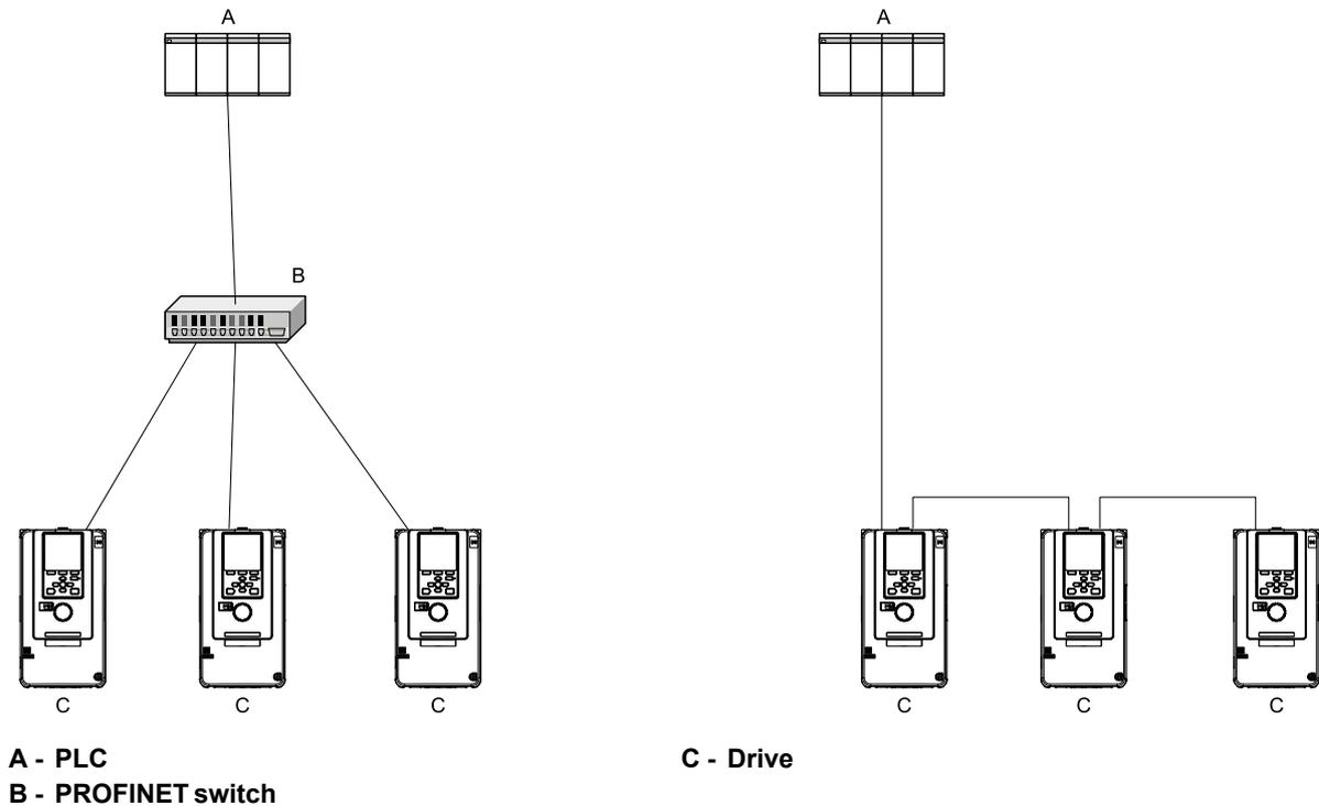
Figure 5.23 Prepare and Connect Communication Cable Wiring
