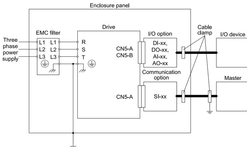
Figure 11.4 Option Installation for CE Compliance: FP605
