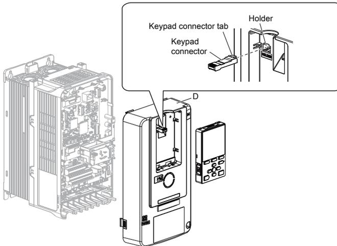
**Figure 5.8 Remove the Front Cover and Keypad**
