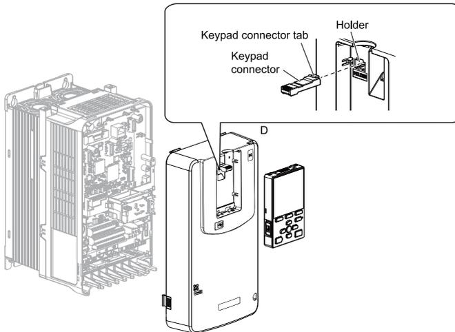
**Figure 5.14 Remove the Front Cover and Keypad**
