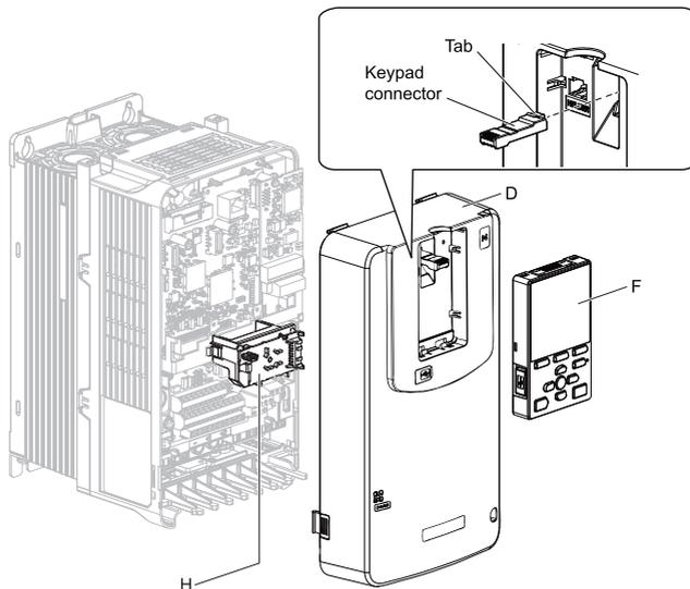
**Figure 5.17 Reinstall the Front Cover and Keypad**
