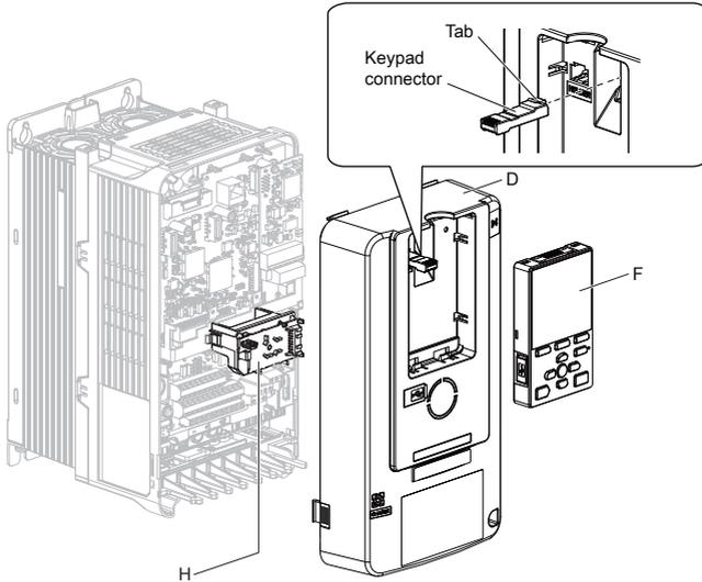
**Figure 5.11 Reinstall the Front Cover and Keypad**
