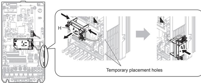
**Figure 5.9 Remove the LED Status Ring Board**
