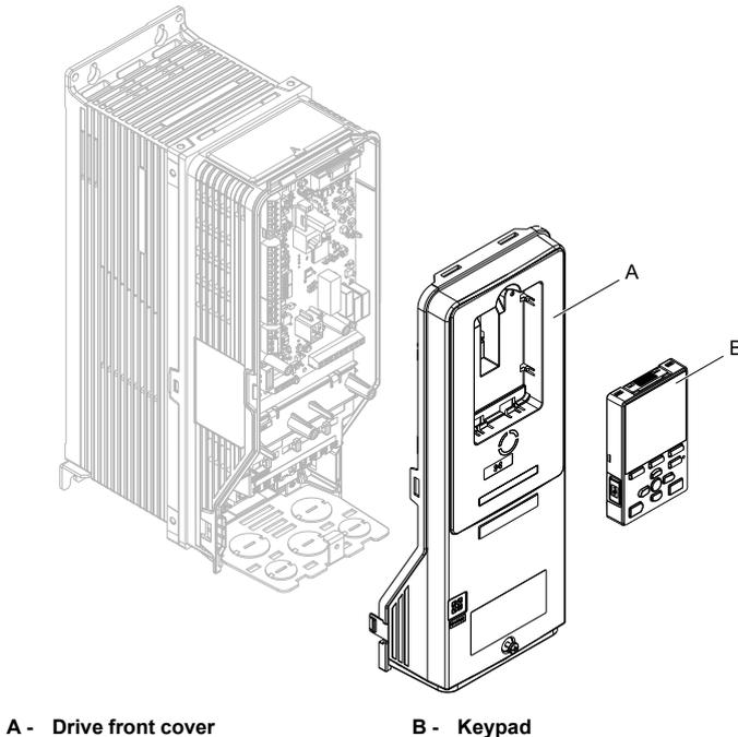
**Figure 5.17 Remove the Front Cover and Keypad**
