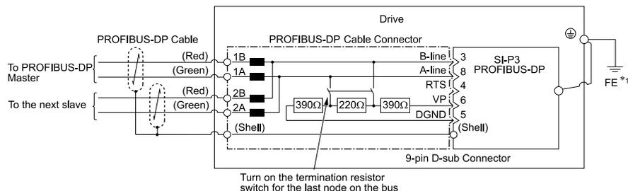
**Figure 5.24 Option Connection Diagram**
