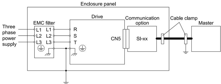
**Figure 10.3 Option Installation for CE Compliance: GA500**
