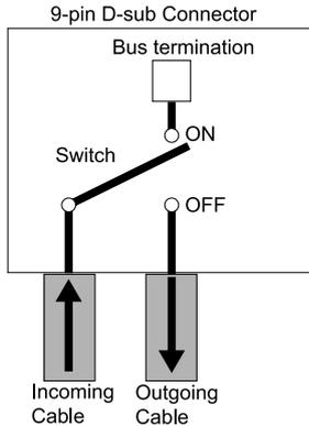
**Figure 5.25 PROFIBUS Cable Connection with Termination Resistors**
