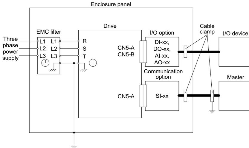
Figure 10.4 Option Installation for CE Compliance: FP605
