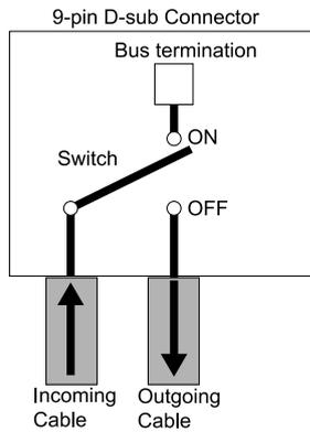
**Figure 5.25 PROFIBUS Cable Connection with Termination Resistors**
