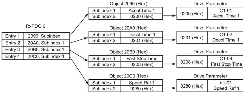
If the PDO contains invalid data, then only the valid data will be written to the drive. Using the example above, if the data for C1-01, C1-09 and d1-01 are valid and the data for C1-02 is out of range, then only parameters C1-01, C1-09 and d1-01 will be changed in the drive, and the data for C1-02 will be ignored.
