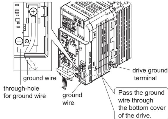
**Figure 10 Ground Wire Connection**
